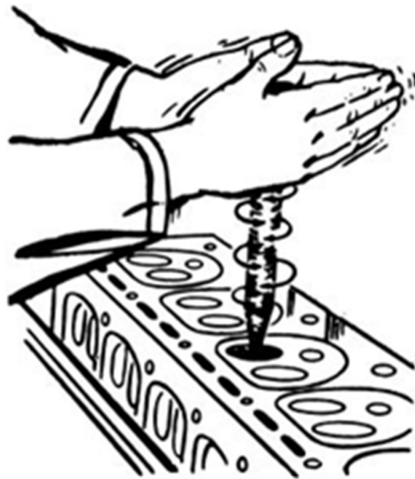
Fig. 2.10: Valve lapping process
