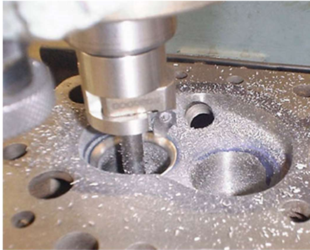
Fig. 2.9: Seat Cutting operation
