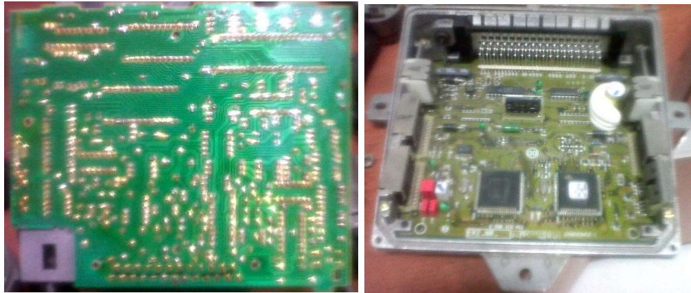
Fig. 2.28: Internal components of ECM
