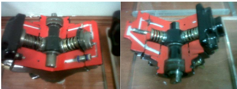
Fig. 2.27: Cut section view of high-pressure pump
